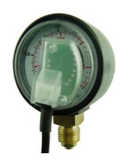
CNG201C is a optical sensor gauge for CNG application, the singal output is in step type, machenical accuracy is ±1.6%, electric output accuracy is ±2.5%. This type of sensor gauge is working with LED switches, or other systems which can treat point signal in volt or resistance.
