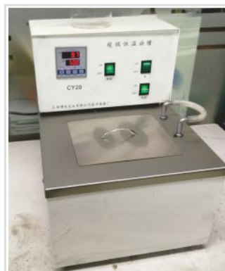
高精度恒温油槽 High accuracy thermostatic oil bath
